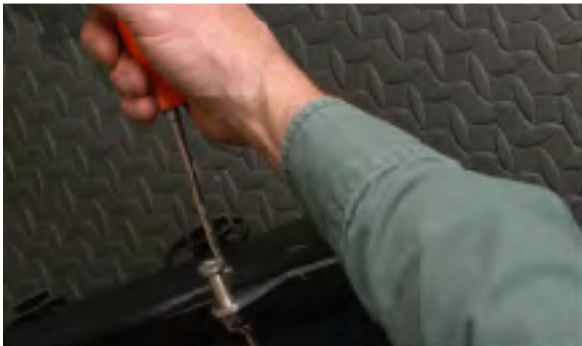
11. With the hardware provided, install three truss head screws (T) through the bag . Place the striker plate over the screws on the inside of the bag and tighten with the acorn nuts (S) provided.
