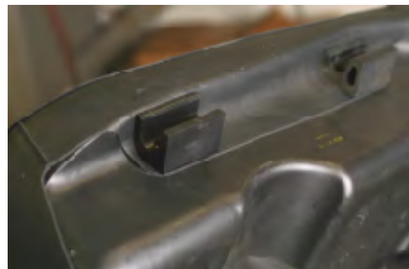
14. Using the hardware provided, bolt the rigid rail clamp (U) in place with the bolt heads (V) inserted through the clamp and the bag. Secure with the acorn nuts (S) provided.
