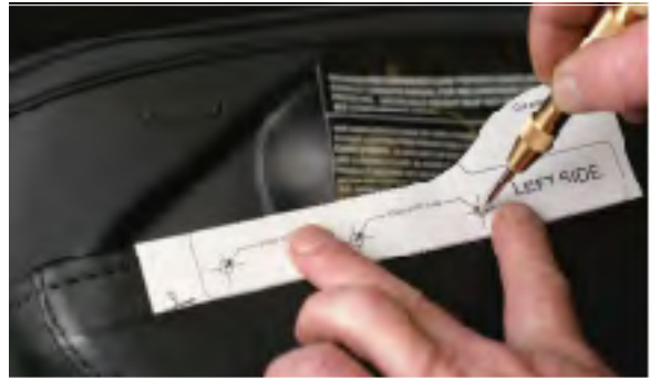
10. Affix the template to match the contour of the bag. Drill the holes as shown on the template.
