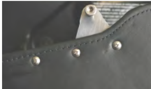
12. Install the striker bolt (R) in the plate with the shoulder bolt head facing out. Tighten in place using the acorn nut (Q) provided.
